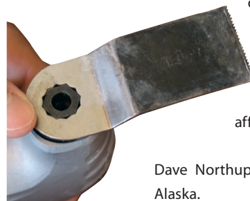
Bosch prevents slippage by keying its blades to a series of pins on the mounting plate (above left). If an adapter (above right) is placed over the pins, Fein's blades can be used on this tool. The 12-sided hole in a Rockwell blade fits over a six-sided post on the tool (right).
