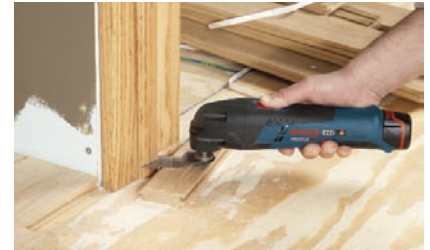
Multi-tools can be used for such tasks such as cutting out drywall (far left), removing grout and excess thinset (left), and trimming door jambs (below).
