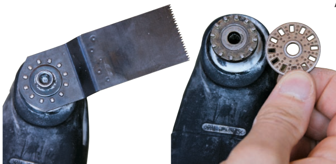
Bosch prevents slippage by keying its blades to a series of pins on the mounting plate (above left). If an adapter (above right) is placed over the pins, Fein's blades can be used on this tool. The 12-sided hole in a Rockwell blade fits over a six-sided post on the tool (right).
